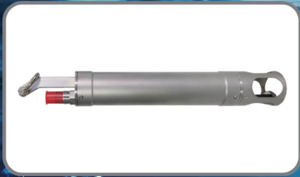
The HY1203 SVP measures underwater sound velocity, depth and temperature where the sensor is for calibrating echosounders, sonar systems and other acoustic instruments. It adopts "Time of Flight" technology and improves the accuracy to 0.05 m/s, which reaches to world-leading level. It is extensively used in the field of hydrography, geophysical exploration, defense and security, scientific research, etc.
